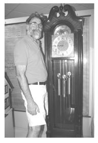
mechanism. The three brass weights that are seen from the front of the glass door are, however, faux; they will never change position, locked for eternity!
